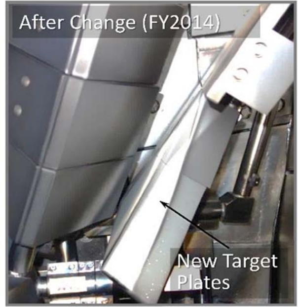
Fig.1 The image -of the carbon-rich mixed material deposition layers on the dome plates in front of the target plates in the original target plate configuration in FY2013 (a) and that in the new target plate configuration in FY2014 (b).
